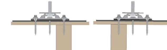
Roof Tech Inc. AlphaSeal™ Technology has been used on over one million residential PV systems since 1994. It is the first PV mounting system with Flexible Flashing certified by the ICC, engineered to withstand wind speeds up to 180 mph and ground snow up to 90 psf.
